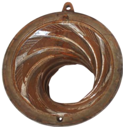
Lining for Simo® grinder before refurbishment
