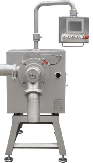
Superpump SP 250 shown below feeding a scanDebone 150.
