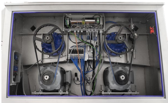
scansteel foodtech® Twin Shaft Mixer, TSM(V) shown with back panel open, view of motors.
