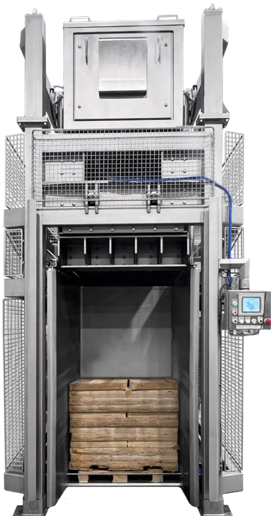
Rear view showing how the frozen pallets are loaded into the Cut the top.
