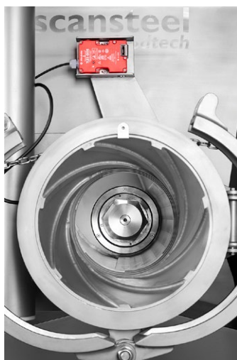
Cabinet without worm/auger showing the flights of the lining.
