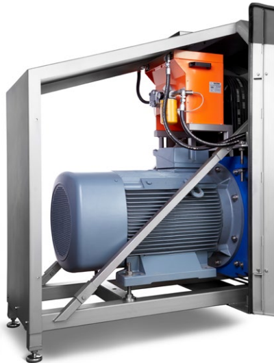
Built-in oil coolers for gear box dramatically increase life time of the gear box.
