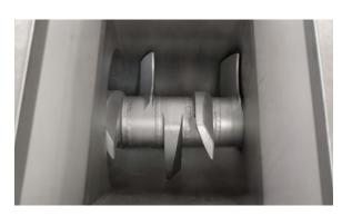
scansteel foodtech \* scanStructor top view, showing the infeed hopper with heavy duty crushing claws.
