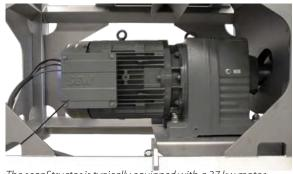
The scanStructor is typically equipped with a 37 kw motor.
