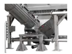
Buffer hopper with mounted weighing cells for batch control and automatic start/stop of machinery.
