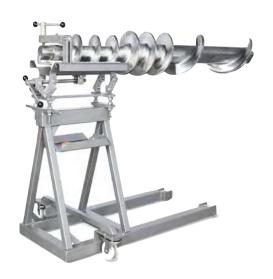
Assembly/ disassembly trolley in stainless steel execution.
