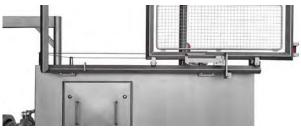
Top picture: Safety guard for platform shown in running position. Bottom picture: Safety guard for platform shown in open/cleaning/inspection position.
