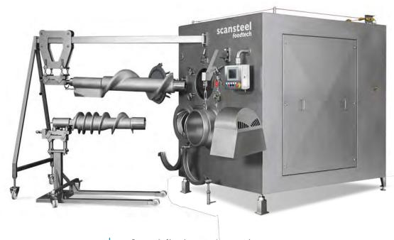
Removal of breaker worm/auger and grinding worm/auger. CombiGrind CG 400 – The Beast
