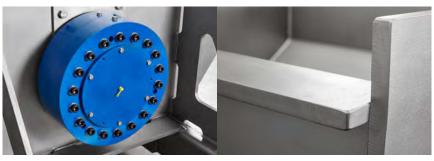
Heavy Duty bearings – on each end of the crusher claw(s). Absorbing/eliminating all axial forces between claw(s) and gear box.
