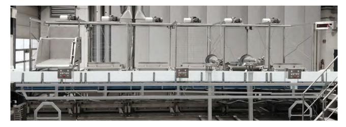
6 (six) unit weighing station, seen from the batching/weighing side. The operator looks at the control panel to the right to check how many kilos he requires of a certain meat raw material. Next, the operator looks at the operator panels in front of each swing loader to see where he has to unload/weigh out the volume of the meat required. The weighing belt is equipped with 4 (four) load cells in order to monitor weights continuously.
