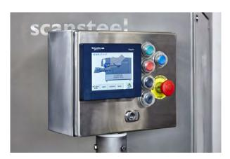
Operator control with easy-to-understand push button operation of start, stop, and emergency. Pre-setting of worm/auger speeds and programming functions with logically designed graphics on the touch panel. Programmes with fixed settings for various products can be keyed in with password protection. The scansteel foodtech® scanControl function can be set to optimize the feeding worm/auger speed in relation to the grinding worm/auger, thus reducing grinding capacity flow fluctuations.
