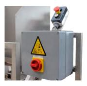
Operator/control panel with emergency stop.
