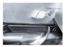
Cheese feed guide shown right mounted. Electro polished feeding worm/auger, also shown.
