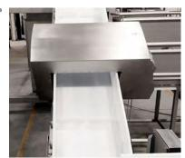
Standard scansteel foodtech® inclined belt conveyor with metal detector, Front top view. scansteel foodtech A/S can deliver our belt conveyors with any brand type metal detector. Front top view.
