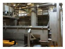
scansteel foodtech® Whole Pallet Crusher, WPC 2000-Single, shown in application where existing footprint is sparse and where the pre-broken frozen blocks must be elevated to approx. 5000 mm.
