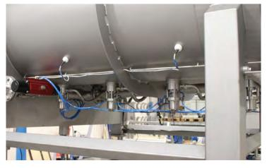
Close up of scansteel foodtech $^\circ$  Bottom steam injection system shown on Twin Shaft Mixer, TSM(V)
