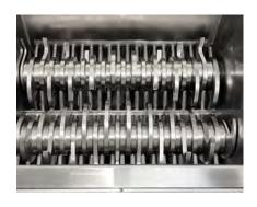
Top view looking at the inside/infeed section where the whole pallets of meat raw material will be fed into the WPC 2000.
