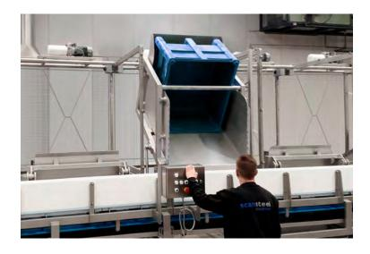
With the scansteel foodtech® line control, it is possible to guide the operator into the exact amount of each meat raw material to be unloaded onto the weighing/batching belt conveyor.
