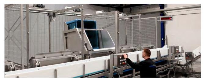
One option in the scansteel foodtech $^{\circ}$  "batching family of solutions" is a station of typically 2-8 swing loaders (tippers) which can hold different meat raw material.
