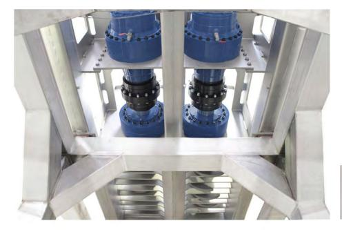
Bottom picture: Please note the shock absorbers which allow the WPC to remain stable (not moving) even when the WPC is fed by a fork lift truck dumping whole pallets into the crusher cabinet.
