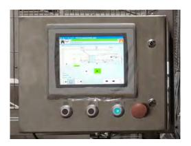
Line control of weighing and batching station.
