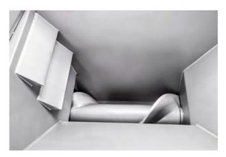
Fresh soft meats as well as tempered or hard frozen blocks are efficiently processed jointly or separately without changing any mechanical components due to the ingenious design of hopper, transfer area between the worms/augers combined with efficient fixation of the frozen blocks. Narrow tolerances eliminate backwash, fines, or smearing.
