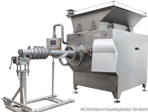
MG 330 shown with optional flange mounted extension infeed hopper and trip wire.
