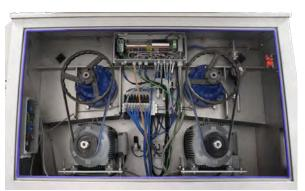
scansteel foodtech<sup>®</sup> Twin Shaft Mixer, TSM(V) shown with back panel open, view of motors.
