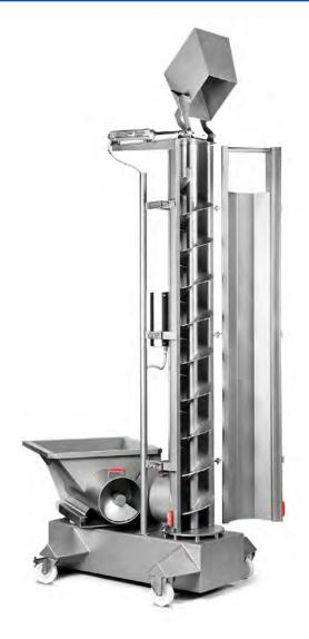
scansteel foodtech<sup>®</sup> standard scanGiraff shown in cleaning position. Note the vertical screw is 100% accessible for cleaning (no hidden zones).
