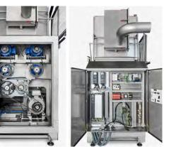
Side panels for easy access to the interior of the machine.
