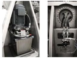
Pallet inverter seen from behind without cover, view of hydraulic unit and turning device.
