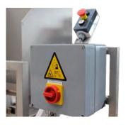
Operator/control panel with emergency stop.
