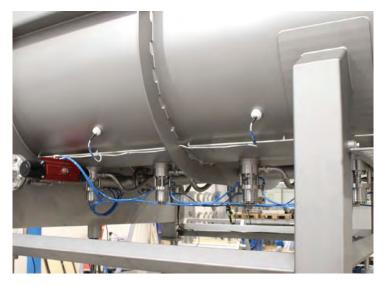
Close up of scansteel foodtech<sup>®</sup> Bottom steam injection system shown on Twin Shaft Mixer, TSM(V)
