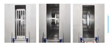
Hygienic zone shown in 3 (three) positions: running position (closed) and cleaning position shown from both angles.
