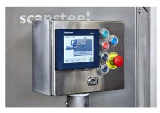
Operator control with easy-to-understand push button operation of start, stop, and emergency. Pre-setting of worm/auger speeds and programming functions with logically designed graphics on the touch panel. Programmes with fixed settings for various products can be keyed in with password protection. The scansteel foodtech<sup>®</sup> scanControl function can be set to optimize the feeding worm/auger speed in relation to the grinding worm/auger, thus reducing grinding capacity flow fluctuations.
