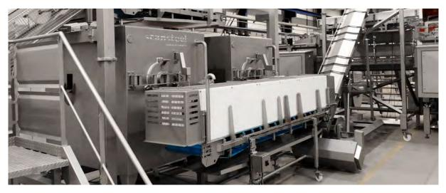
Another typical horizontal belt conveyor solution where 2 (two) grinders are discharging onto the scansteel foodtech<sup>®</sup> belt conveyor. This solution saves a lot of safety devices and, at the same time, secures easy access to the grinders for cleaning, mounting, and dismounting of the grinders, front view.
