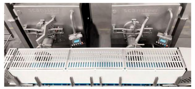
Another typical horizontal belt conveyor solution where two grinders are discharging onto the scansteel foodtech<sup>®</sup> belt conveyor. This solution saves a lot of safety devices and, at the same time, secures easy access to the grinders for cleaning, mounting and dismounting of the grinders, top view where the transfer point from grinders to belt conveyor is clearly seen.
