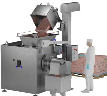
The scansteel foodtech<sup>®</sup> MG 225 is designed to be fed by either a belt conveyor or a lifting, here shown being fed by the scanLift SC 350 with 220 L trolley.
