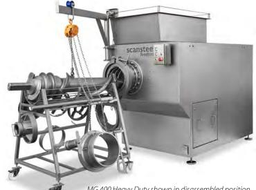
MG 400 Heavy Duty shown in disassembled position and with all loose parts positioned on accessory/ cleaning trolley for inspection and cleaning prior to assembly.
