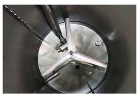
Mixing container designed for heavy viscous gravies/ mixtures. The Ytron and the Venturi system in combination with the Heavy Duty mixing agitators ensure a fast processing of a gravy free from lumps. Anti-vortex breakers are standard in all scanGravy mixing tanks. Direct steam injection for temperature control can be added as well.
