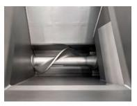
Top view of infeed hopper of the MG 225
