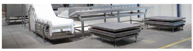
Belt Conveyor with unpacking station with 2 (two) lifting tables for ergonomics, left side.
