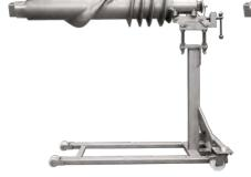
Cleaning trolley for worm/auger shown after the worm/auger has been removed from grinder.
