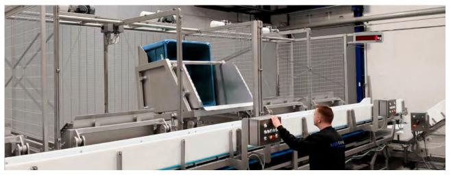
One option in the scansteel foodtech<sup>®</sup> "batching family of solutions" is a station of typically 2 – 8 swing loaders (tippers) which can hold different meat raw material.
