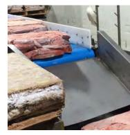
The scansteel foodtech® Inclined Chain Bulk Conveyor is designed with a pitch chain system in each side of the bulk conveyor and equipped with stainless steel guides/flights for transportation of the product. The Inclined Chain Bulk Conveyor can be equipped with infeed chute if used in combination with other belt conveyor installations.
