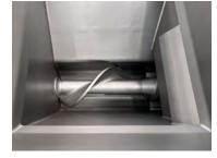
Top view of infeed hopper of the MG 225
