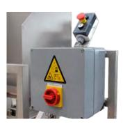
Operator/control panel with emergency stop.
