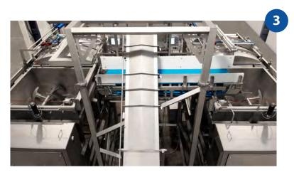
Close-up view showing scansteel foodtech® inclined screw conveyor feeding onto a scansteel foodtech® horizontal belt conveyor which has 3 (three) main positions.
