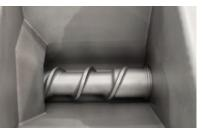
View of hopper infeed of MC 300 - Hopper fed
