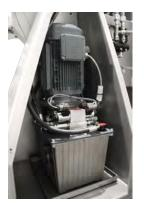
Pallet inverter seen from behind without cover, view of hydraulic unit and turning device.
