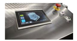
Electrical panel, including touch panel and manual buttons. The cabinet is certified stainless steel, AISI 304 execution.
