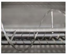
Top view and inside look of the TSF. Both the twin screws Close up view of twin screws, top view. and the feeding wing is shown.
