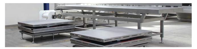
Belt Conveyor with Unpacking station with 2 (two) lifting tables for ergonomics, right side.
