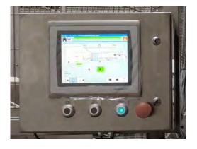
Line control of weighing and batching station.
