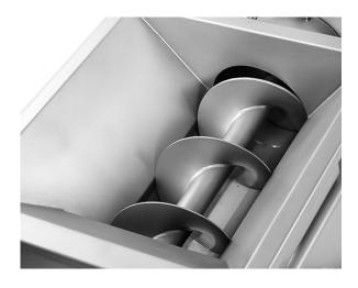
Large diameter infeed screw in horizontal infeed hopper.
